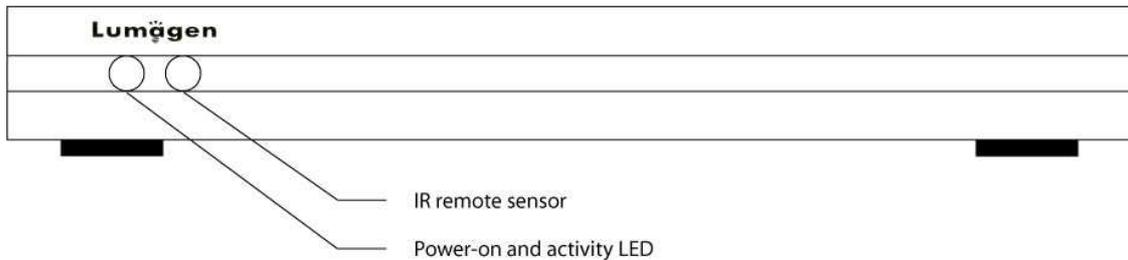
The front panel has a light-emitting-diode (LED) indicator, which is red when the unit is in "standby" and, by default, is green when the unit is "on." Note that the green "on" indicator can be turned off if preferred.
