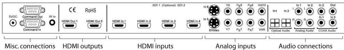
There are four HDMI and six analog video inputs. Audio can be received on the active HDMI input, one of two analog stereo inputs, or one of five digital audio inputs (2 TOS, plus 3 COAX).
