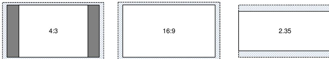
Figure 1, 16:9 projector with fixed zoom used on a 2.35 screen
